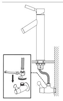
Connect hot and cold waterlines (8) to the angle stops and tighten with a wrench. Unscrew the aerator cover by hand, and remove the aerator, then turn on the water to remove any leftover debris
