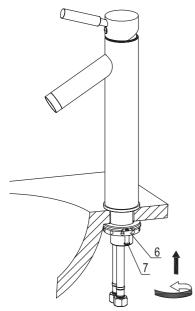
After adjusting the direction of the faucet body (1), tighten the mounting nut (6) until snug and then tighten the mounting screws (7) to the nut with a Phillips head screw driver until snug.
