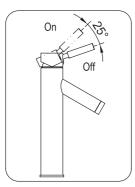
Raise the lever handle to turn on the water. Push down to turn off.
