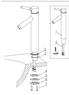
Screw and hand-tighten the hot and cold waterlines (8) into the faucet body (1), hot side left & cold side right when spout is facing up. Install the faucet body (1) through the 1-3/8" predrilled hole in the countertop. Attach the rubber washer (4), metal washer (5), mounting nut (6), and mounting screws (7) from underneath the sink.
